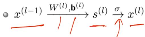
The diagram illustrates the forward pass of a specific layer in a neural network. It shows the input vector  $x^{(l-1)}$  being multiplied by the weight matrix  $W^{(l)}$  and the bias vector  $\mathbf{b}^{(l)}$  to produce the sum  $s^{(l)}$ . The sum  $s^{(l)}$  is then passed through an activation function  $\sigma$  to produce the output  $x^{(l)}$ . Red arrows indicate the flow of information from left to right, with a red arrow pointing up to the activation function  $\sigma$ .
