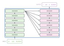
The Encoding module has a stack of encoders
